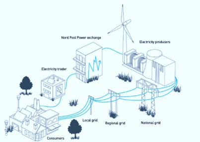
The diagram above shows the route of electricity from the producer (power station) via the national grid, regional network, local network and finally to the electricity consumer. The producers sell their electricity on the Nord Pool power exchange or to electricity suppliers. Suppliers sell the electricity on to the consumer.
